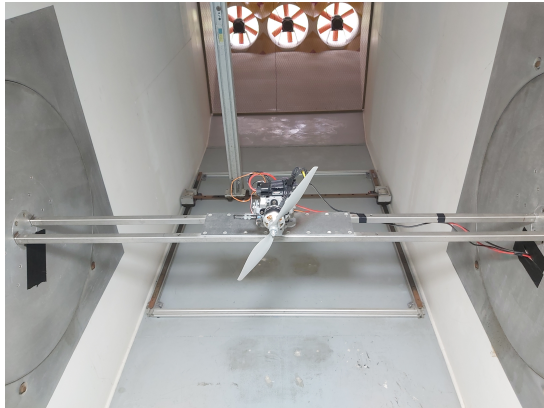
Figure 14. Setup integrated in wind tunnel.
